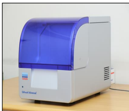
QIAxcel (Capillary Electrophoresis)
