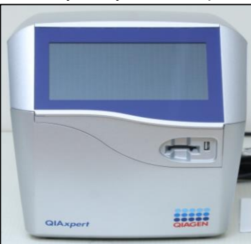
QIAxpert (Microfluidic UV/VIS Spectrophotometer)
