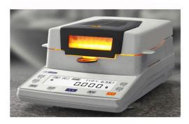
Moisture analysis is the method used to measure the percentage of water in the sample.
